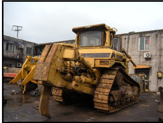
Photo 1. Bulldozer fitted with tooth at rear for 'ripping'
